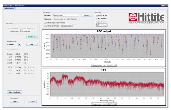
Figure 29.EasySuit view showing the effects of too much gain and saturation
