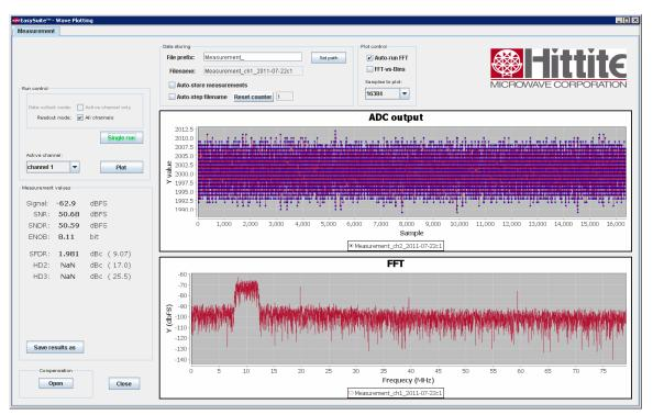
Figure 23. Observed result after 20 dB of gain in the first VGA
