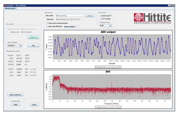
Figure 37. System View dialog showing the effect of increasing the filter bandwidth to 7 MHz
