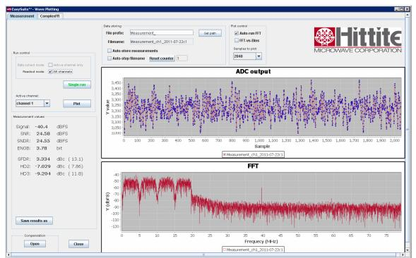
Figure 52.DCR EasySuite measurement window showing received 4 carrier WCDMA signal FFT and time domain
