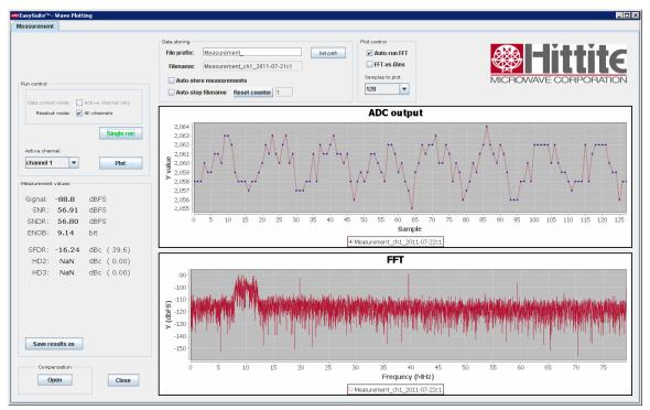
Figure 20. Resulting EasySuite Measurement View
